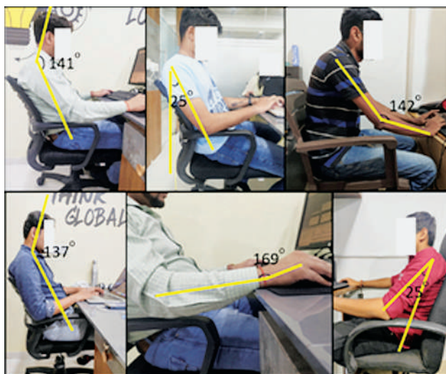
Fig. 3: Assessments done for calculating postural angles using Imagej Software.
