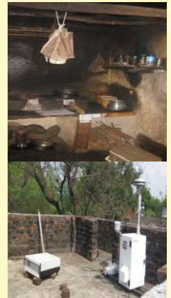
Integrated indoor and outdoor PM 2.5 area measurements
